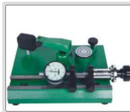
Inspect accuracy of dial indicators (range 0-25mm)
