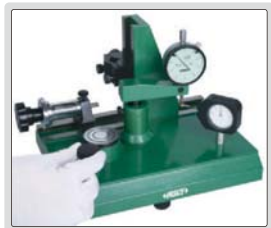
Test force of dial indicators
