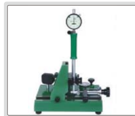
Inspect accuracy of dial bore gages (range 0-450mm)
