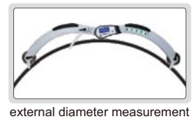
external diameter measurement
