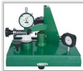
Test repeatability of dial indicators
