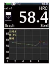
Graph display mode, show average value, relative range and test times
